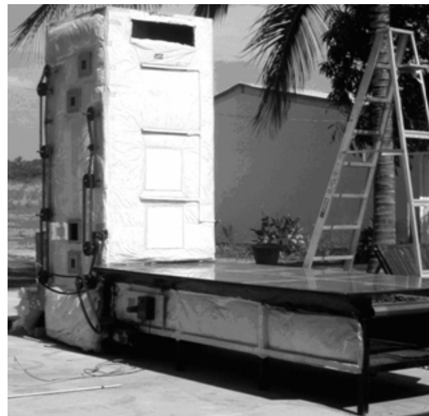
Fig. 6. Picture that show the real solar drying system for Roselle and other products
