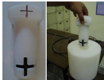
Figure 6. Plug, and plug being inserted on moderator
